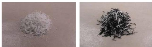
Fig.6 Appearance of silica ashes prepared by burning citric leached rice husk (a) and as-received one (b).
