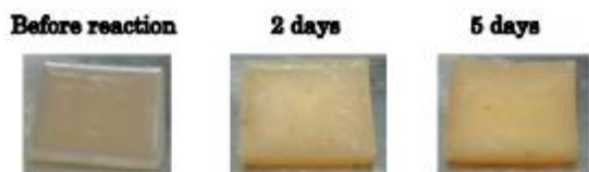
Fig. 10. Result of immersing the mixed resin M2 in 5% acetic acid was heated (pH2.33) to 95 °C
