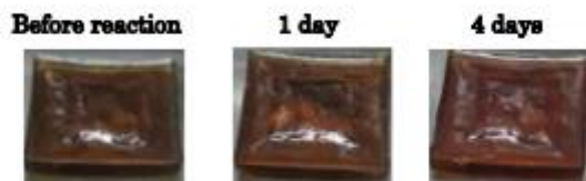
Fig. 8b a result of immersing the mixed resin X 5% acetic acid was heated (pH0.2) to 95 °C
