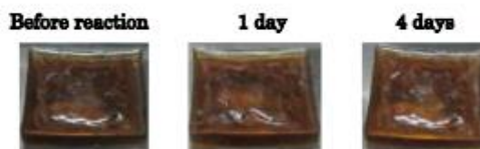
Fig. 8a Result of immersing the mixed resin X 5% acetic acid was heated (pH2.3) to 95 °C
